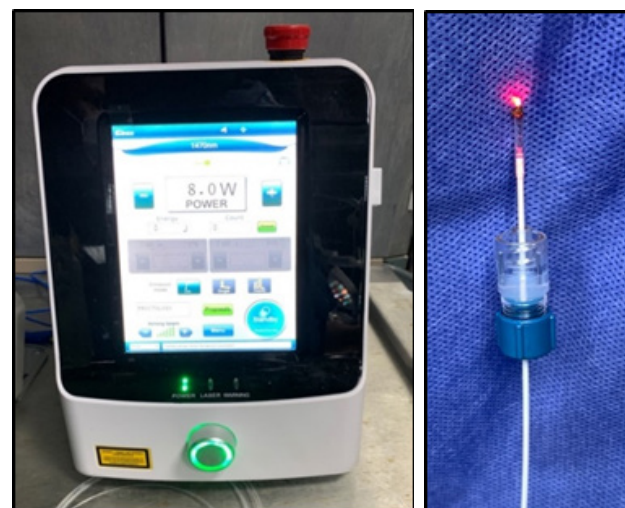
Fig. 1: GigaLaser diode laser demonstrating a power of 8 W, with the bare fiber probe.
