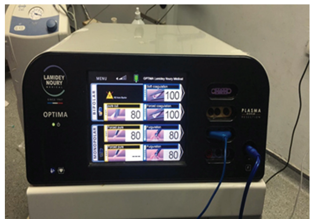
An electrosurgical device with an option of precise pure and various cutting and coagulation modes (we preferred the pure auto-cut mode (good synchronous both cutting and coagulation). Lamidey Noury Medical, Optima generator, France (a new device which can deliver monopolar, bipolar, plasma energy with different modes).
